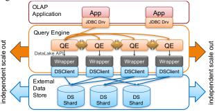
Figure 3. Generic architecture extension for accessing external data
